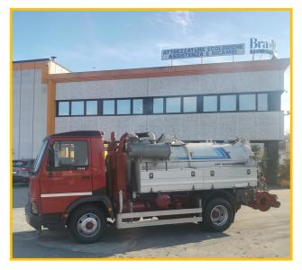
NASPO POSTERIORE LATERALE MANUALE CON 60 METRI DI TUBO ALTA PRESSIONE DA 1/2" + NASPO LATERALE MANUALE CON 60 METRI DI TUBO ALTA PRESSIONE DA 3/8"
